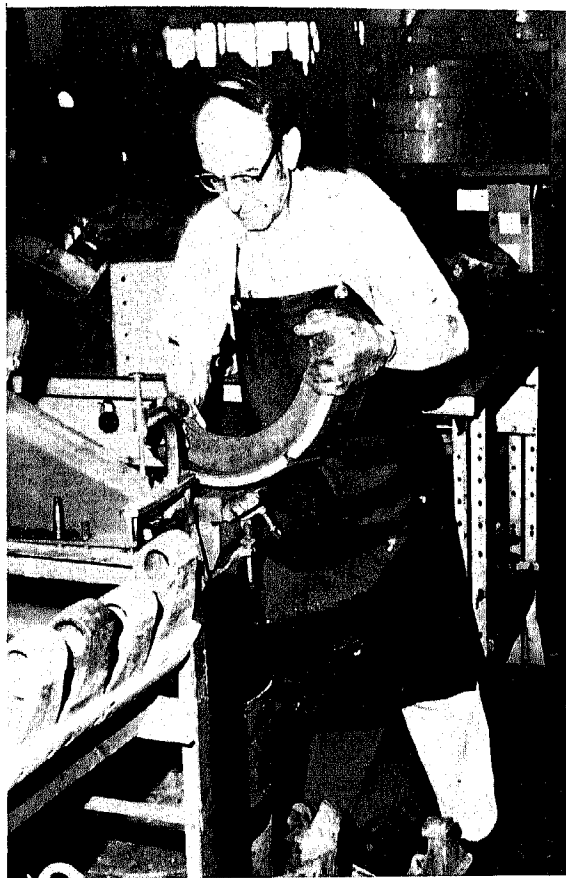
FIG. 6. Renewing of municipal truck brake linings by light grinding to remove grease and dirt.
