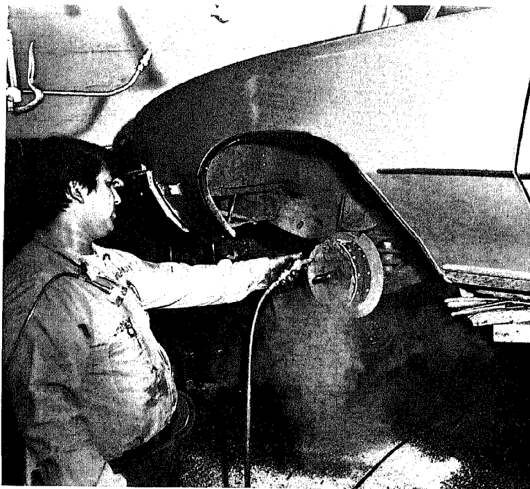
FIG. 4. Removal of dust from brake drum and back plate by pneumatic air blowing at automobile garage.
